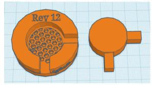
the contact strip extending downward in this view. Then, a sheet of porous carbon paper is laid over that to protect the electrode from damage of the woven character of the screen. The cathode, separator and anode are then laid over the carbon in that order. Next is another "lollypop" shaped current collector made of thin brass that has been heavily gold plated.
